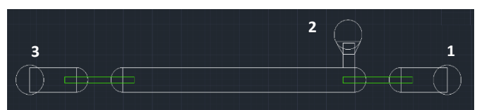
Figure 7 – AutoCAD mask designed by Master's student Pedro Monteiro. The structure has one liquid inlet (1), one beads inlet (2) and one liquid outlet (3).
